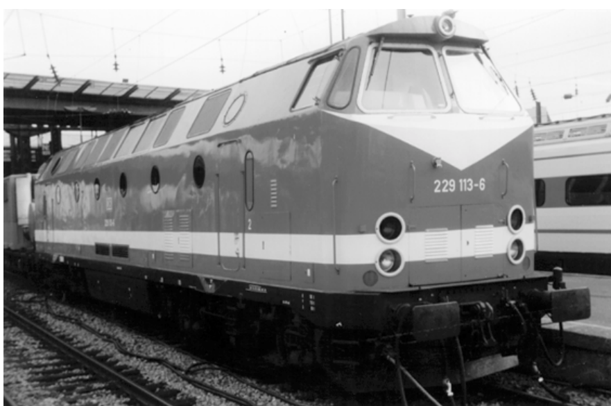
This Class 229 2760 kW DB AG diesel locomotive was built in 1992. Diesel traction still accounts for a considerable part of freight traffic in Europe, although most units are over 30 years old. (Author)
