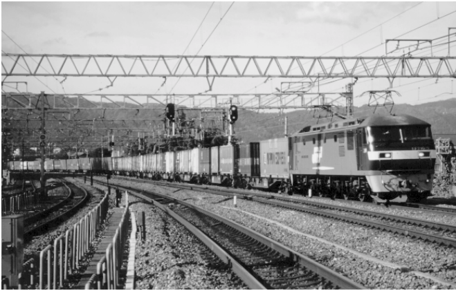
Class EF210 electric locomotive hauling high-speed container train on Tokaido Line (Author)
