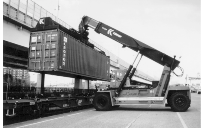
Loading 40-ft international maritime container on Koki 106 container wagon (JR Freight)
