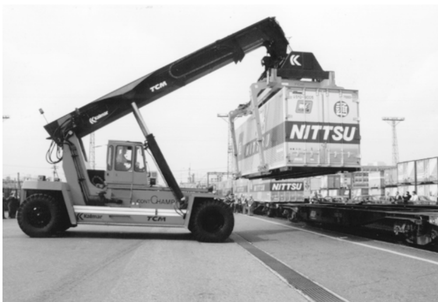
Loading Swap Body at Tokyo Freight Terminal
