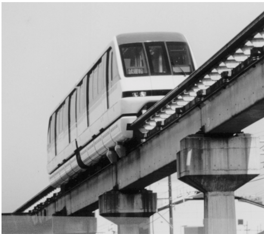
HSST-100L vehicle on elevated test track in Nagoya City
