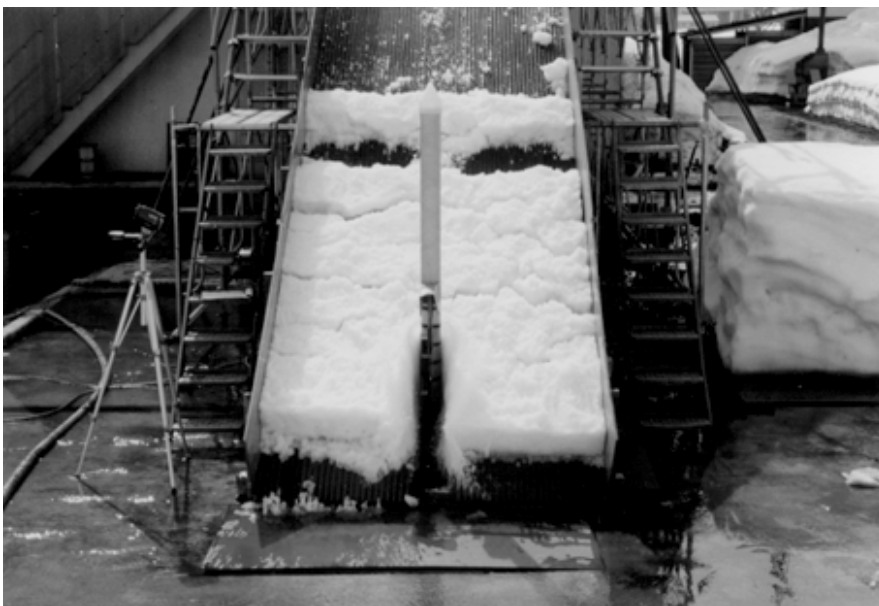
Testing avalanche detection and alarm system at Shiozawa Snow Test Site. Pole in middle for avalanche detection (RTRI)
