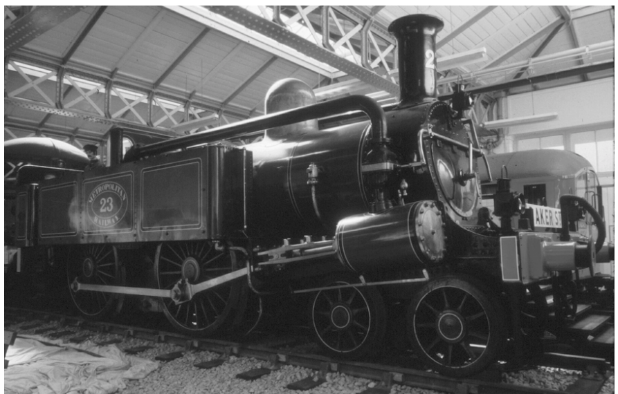
Old steam loco of Metropolitan Railway (built in 1866 by Beyer, Peacock & Co.) with smoke and steam recycling apparatus, preserved at London Transport Museum (EJRCF)
