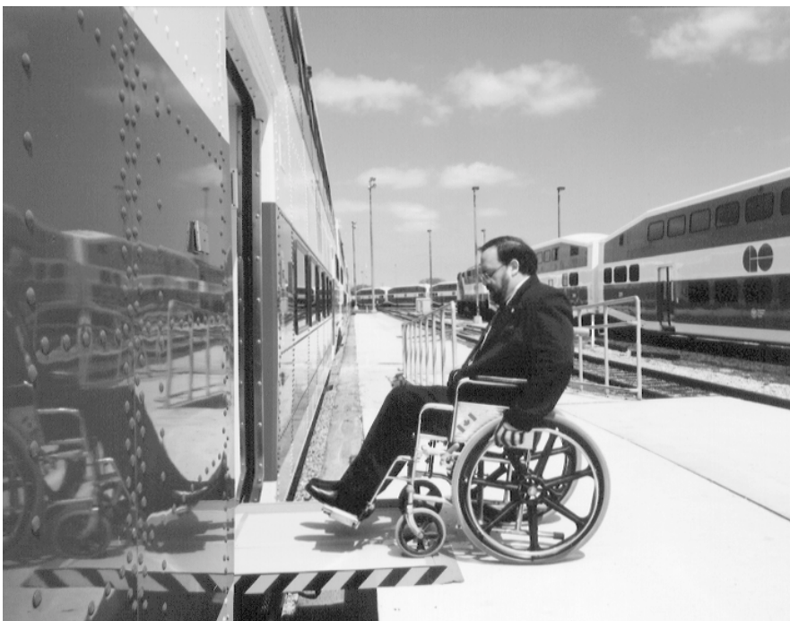
Wheelchair users can gain easy access to carriages across a bridge from the mini-platform.
