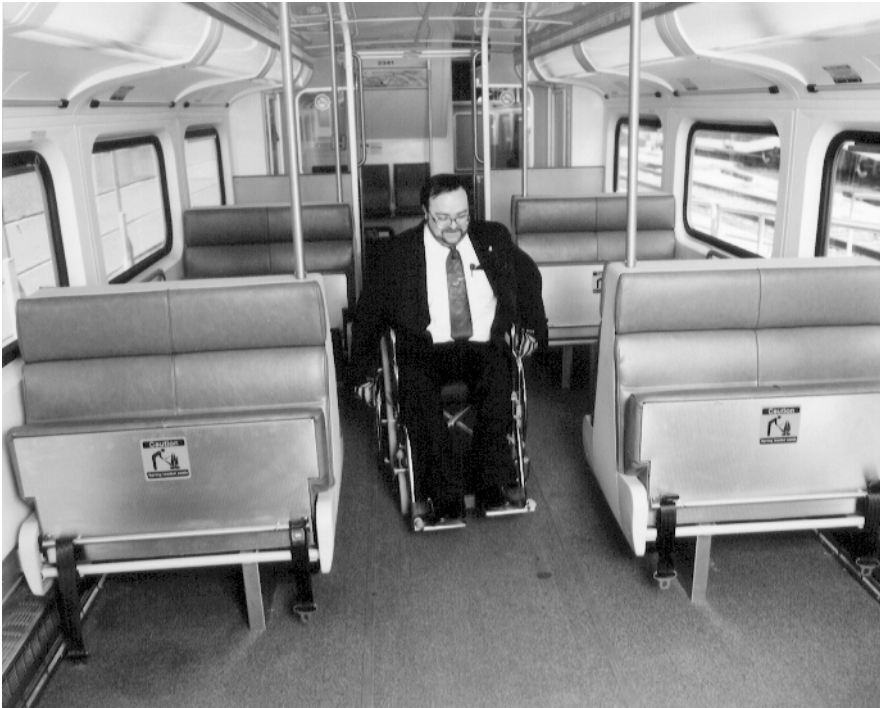
The lower deck of accessible cars has eight wheelchair positions that are easily reached. (GO Transit)
