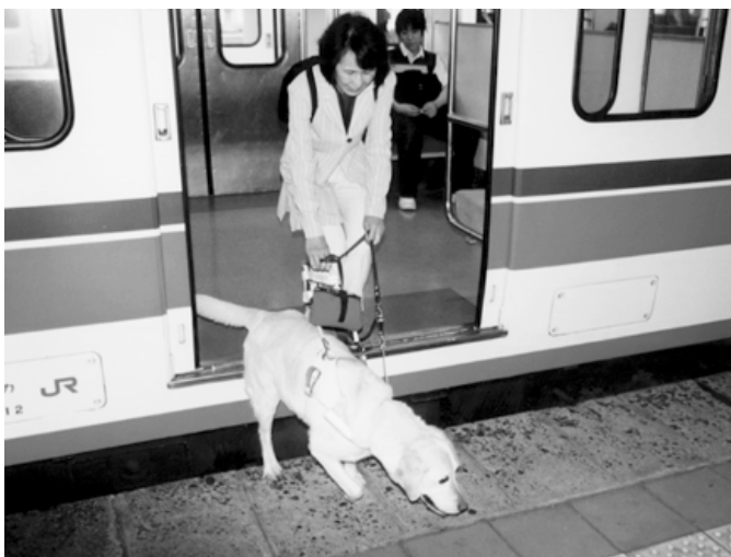
The gap and different level between the train and platform is a serious safety hazard. (Author)
