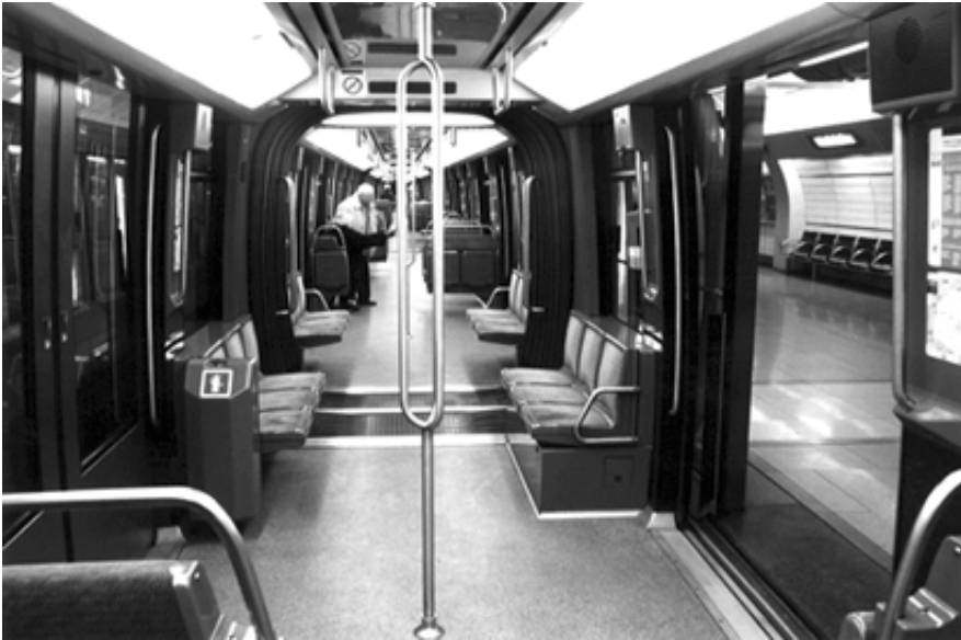
The Paris Météor metro has almost no platform gap.
