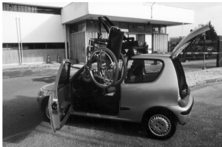
Compact Fiat with roof-mounted wheelchair lift (Portuguese Ministry of Equipment, Planning and Territorial Administration)
