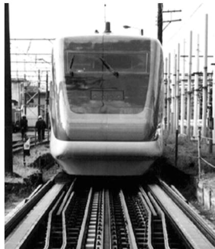
RTRI Experimental free-gauge train passing gauge-changing section on experimental track in Kokubunji, Tokyo (RTRI)
