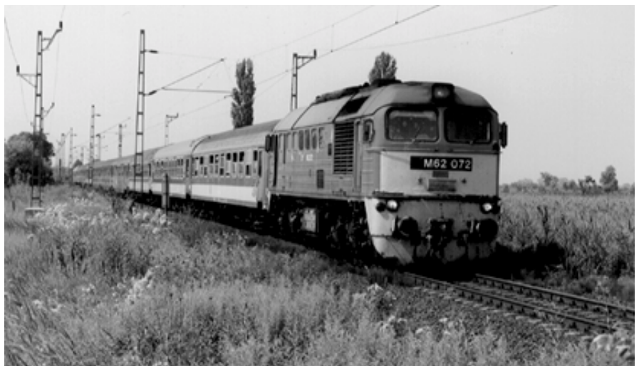
Class M62 diesel loco of MÁV hauling passenger carriages on electrified track
