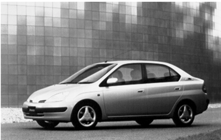
The Prius hybrid car uses both a conventional gasoline engine and a battery-driven electric motor. (Toyota Motor Corp.)
