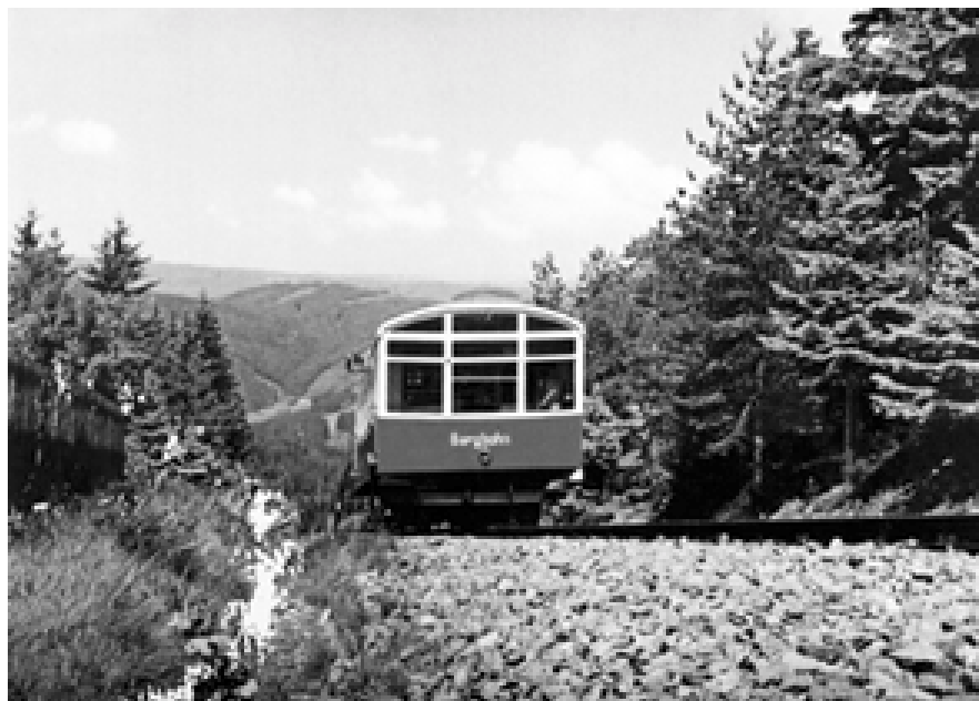
The Oberweissbacher Bergbahn in the Thuringian Forest is a wide-gauge cable car railway climbing 323 m and able to carry standard-gauge freight cars. (DB AG)
