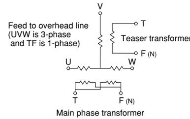
**Figure 6 Modified Wood-bridge Connected Transformer**
