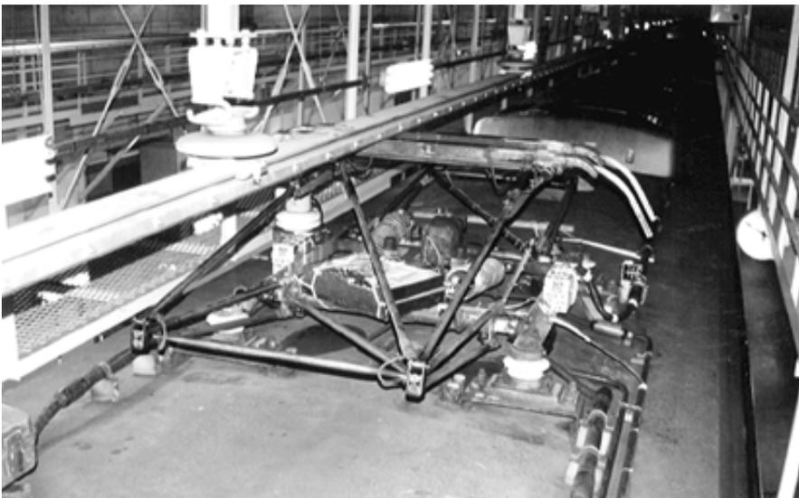
Overhead rigid conductor system and pantograph
