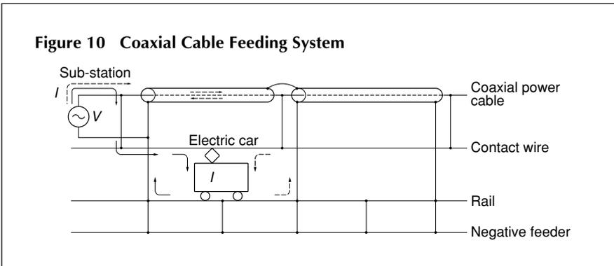
layout is simple, making it ideal for use where space is limited. Japan is the only country that uses this system (the Tokyo sections of the Tohoku Shinkansen and Tokaido Shinkansen).
