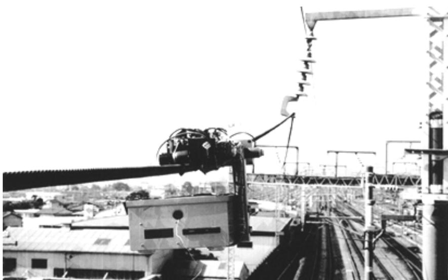
Feeder line inspection robot
