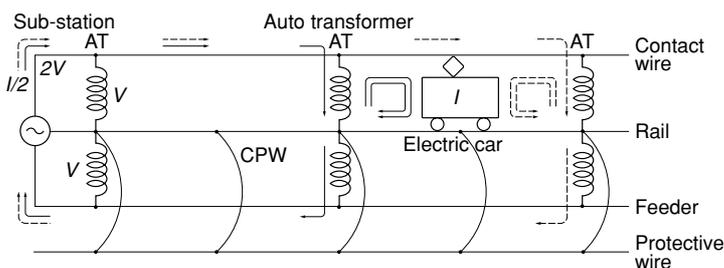
tive feeder to compensate for the reactance and reduce the amount of current intercepted by the pantograph, thereby reducing arcing, and also helping to prevent voltage drop.
