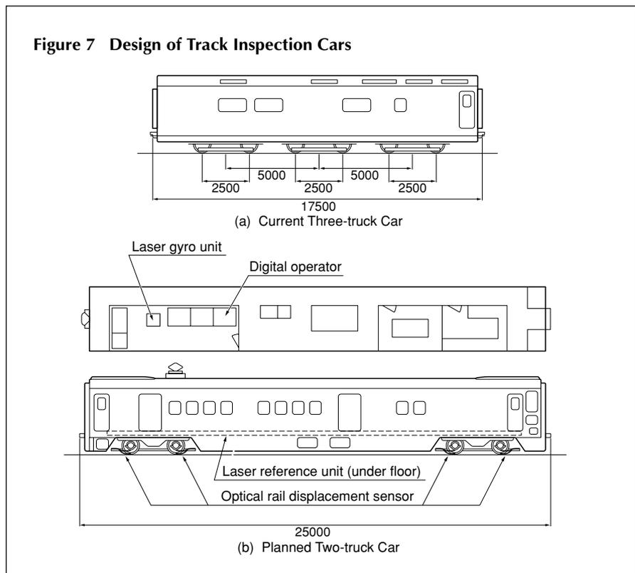
speed in the range of 300 km/h, approaching that of commercial trains. The new inspection car uses three of its four axles to obtain data that are converted to similar data to those obtained by the earlier three-truck car. It also features laser-based equipment, a lightweight optical sensor
