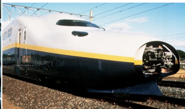
Nose cone opens to couple two trainsets
