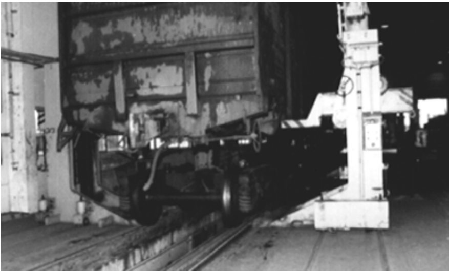
Lifting jacks for changing bogies
