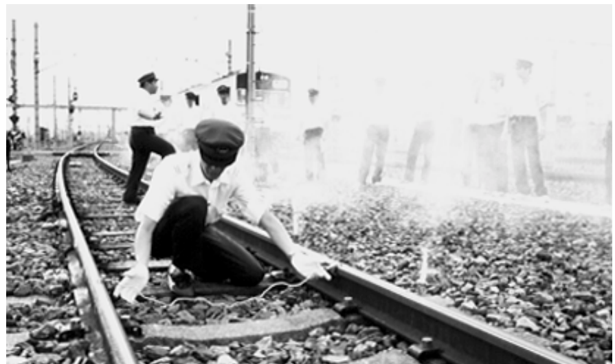
Setting warning flares and track jumper cable to stop oncoming train in emergency
