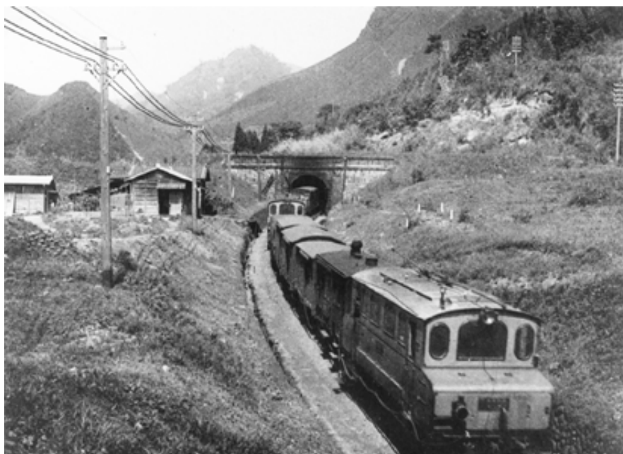
Class 10,000 AEG/Esslingen electric locomotive on Usui Toge Railway
