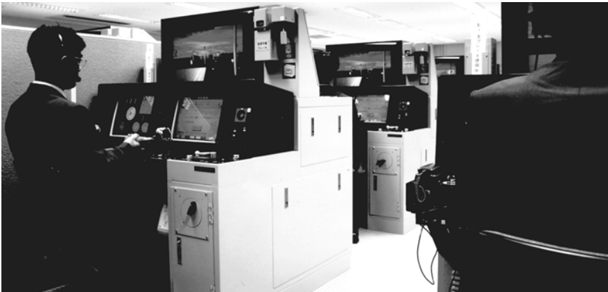
Personal Driving Simulator at JR East Central Training Centre
