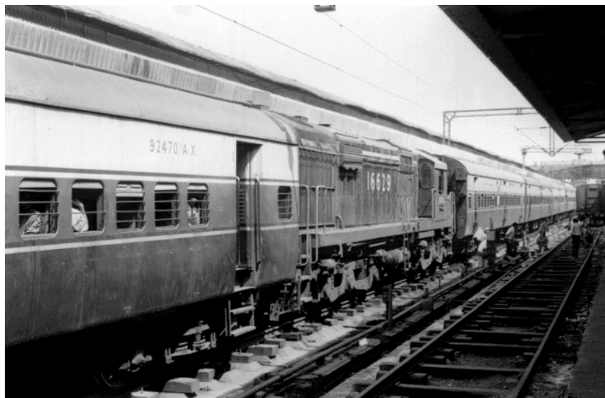
2600-hp Diesel Electric Locomotive in Middle Providing Acceleration Comparable to EMU
