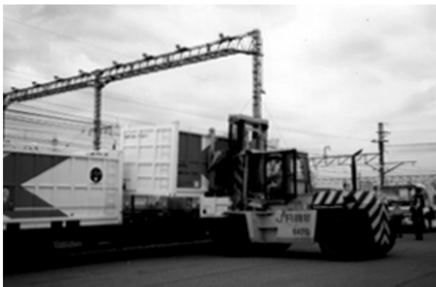
Loading Garbage Collection Container
