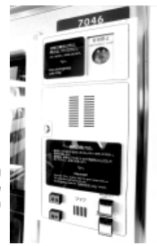
■ Train interphone allowing direct conversation with the central control room in emergency.
