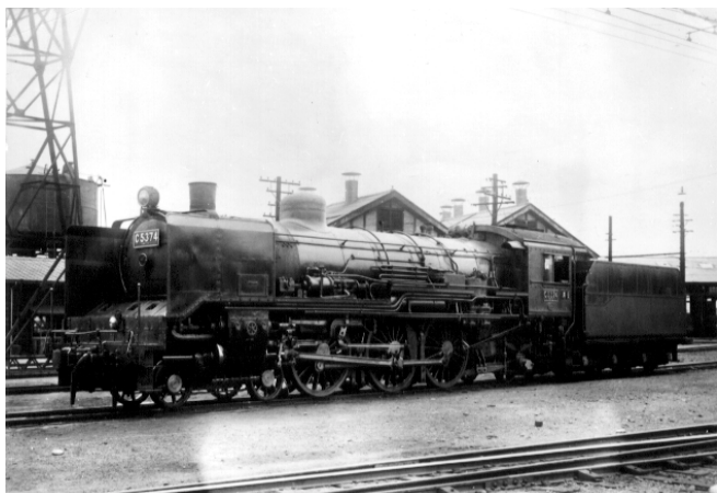
■ Japanese-built 3-cylinder passenger locomotive Class C53 for Tokaido Line express service (1928) (Transportation Museum)
