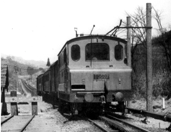
■ German-built first electric Class 10000 Locomotive (EC40) used on Rack-and-Pinion Line (1912) (Transportation Museum)
