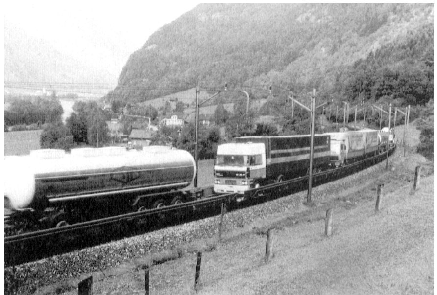
■ Combined Transport at Lötschberg
